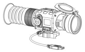
FIGURE 2-6. EXTERNAL BATTERY CONNECTION
